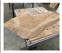
Sand the wood with 120-grit sandpaper so the epoxy will bond with the wood.
