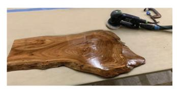
Apply a thin coat of mixed epoxy to seal the wood. This important step prevents air in the wood from off-gasing and creating air bubbles once you've poured epoxy over it. Seal the wood with two thin coats of mixed epoxy, and allow to dry.
