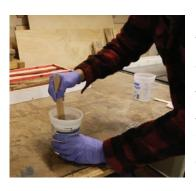
Dispense 1 part resin to 1 part hardener (by volume) into a clean mixing cup. Mix both componnets together thoughly. Mix enough epoxy to pour one layer at a time, at maximum recomended depth of 1/2 inch.
